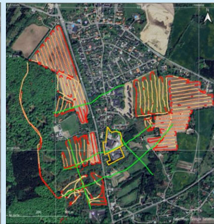
Overview of the investigated area. Red shows tTEM survey lines, yellow shows tTEM data used in the inversion, and green shows DCIP survey lines.
